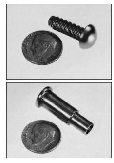
By comparison, steel or copper alloy studs for joining stainless steel would accelerate corrosion of the fastener system, although the extent of the galvanic attack would depend upon the relative area of each material.
