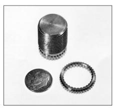
est-strength thread, however, is achieved by thread rolling. This is because the plastic deformation—or cold working involved in rolling threads results in; (1) more accurate and uniform thread dimensions, giving a better fit between threaded parts and fewer concentrated loads at points of misfit; (2) smoother thread surfaces and, thus, fewer scratches and other markings to initiate cracks, or galling; and (3) higher yield, tensile, and shear properties to better withstand ser-
