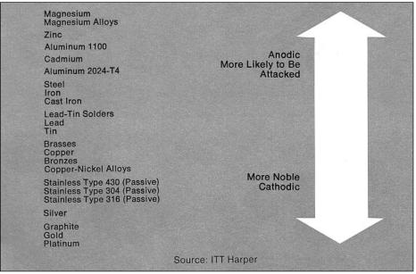
current to flow with corrosion occurring at the anodic component of the cell. Figure 5 provides a guide to the relative anodic and cathodic relationships of metals to
