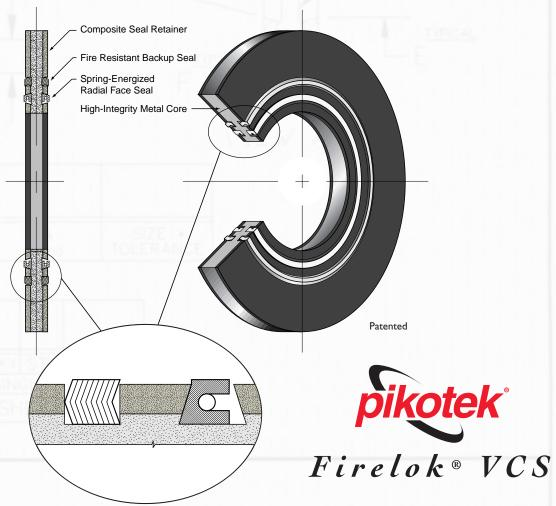
Flowlok/Firelok gaskets and seals are designed for use in all standard ANSI/ASME and API flange types (raised-face or RTJ) and pressure classes and meet all ASME Boiler and Pressure Vessel (BPV) code allowable flange/bolt stresses and B31 piping code requirements as well as API specification 6A dimensional and Appendix F
